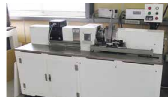
トルク測定器(大型) Torque measurement for large goods.
