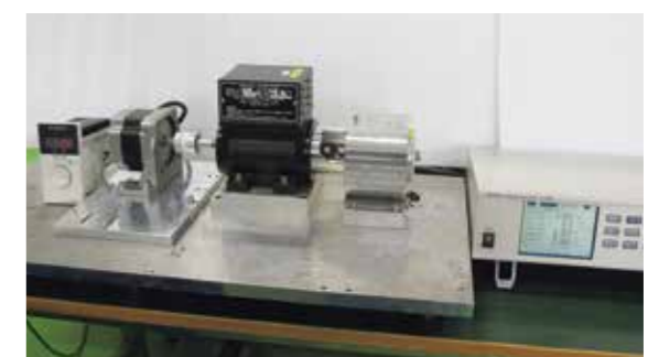
トルク測定器(標準) Torque measurement for standard goods.
